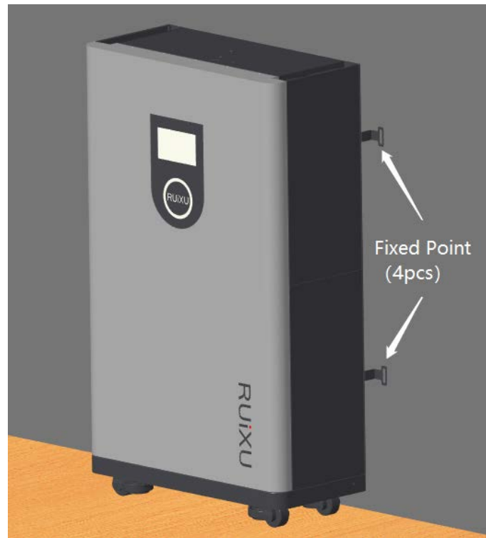
Battery fixation diagram (Installation torque: 9N)
